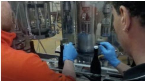
Manual capping with modified screw-cap unit
